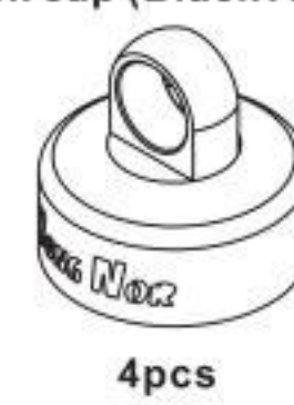
#387C-BK 16mm shock cap (Black Anodize)
