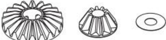
X3-03 Diff. Gear 10Tx4, 20Tx2, 0.15mmx4
