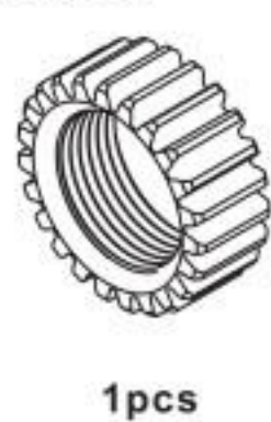
#429H Clutch Gear (2st) 23T
